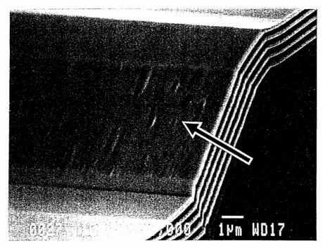
Figure 12 Bird's eye views of the (112)A sidewall layers (indicated by arrow) on (a) the (111)A and (b) (001) patterned substrates. -40
