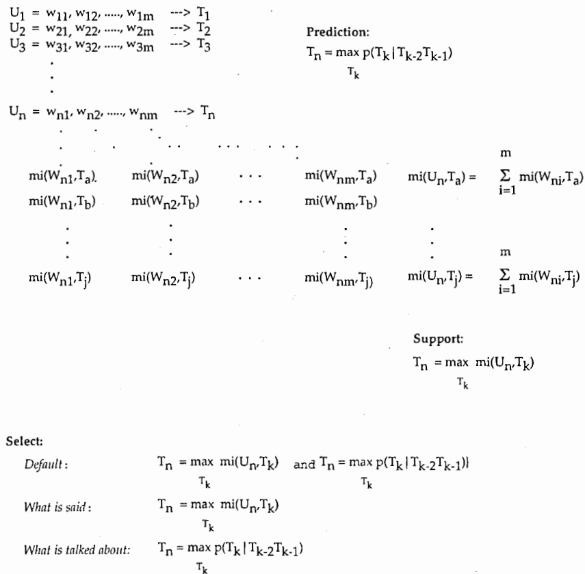
Figure 5: Scheme of the Predict-Support Algorithm.
