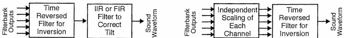
Figure 4. Two approaches are shown here to invert the filterbank. The left diagram shows the normal approach, the right figure shows a more efficient approach where the spectral-tilt filter is converted to a simple multiplication.
