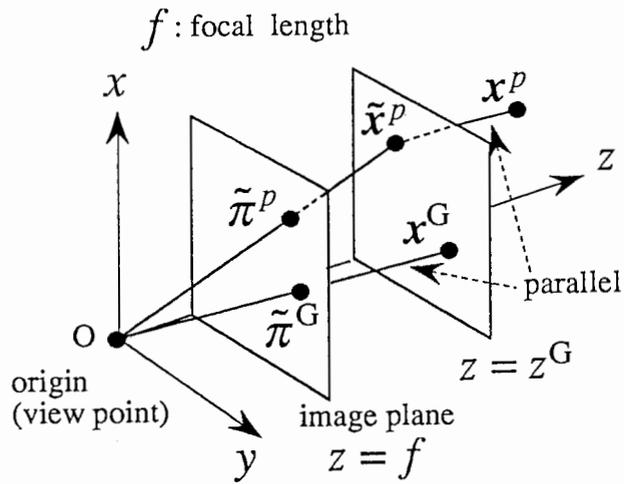
Fig. 1: Principle of paraperspective projection
