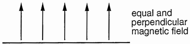
Figure 2.5: Simple model of magnetic attraction on a plane
