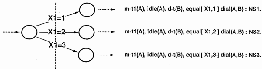
Figure 10.1: The state transition for STR screening rules
